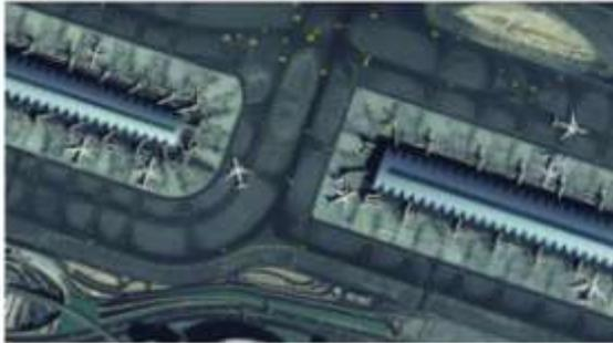
The **DEIMOS-2** provides 75-cm pan-sharpened imagery and 3-m multi-spectral images. Its multi-spectral capability includes 4 channels (**red, green, blue, NIR**), plus the **panchromatic band**. It is the **highest-resolution fully private satellite in Europe**, and one of the very few privately-owned submetric satellites in the world.
