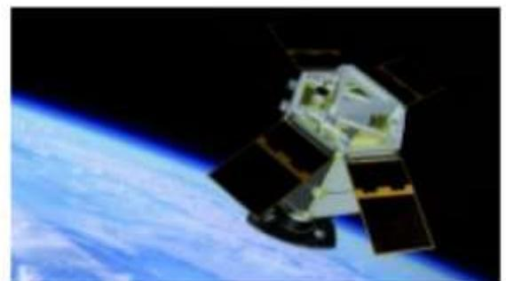
The **DEIMOS-2** provides 75-cm panchromatic imagery and 3-m multi-spectral images. Its multi-spectral capability includes 4 channels (**red, green, blue, NIR**), plus the panchromatic band. It is the highest-resolution fully private satellite in Europe, and one of the very few privately-owned submetric satellites in the world.
