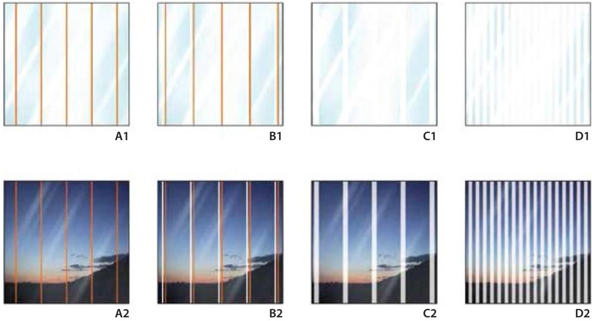
Figure 19.1. Diagram showing various types of vertical stripes for roadside screens. The colours must ensure maximum contrast with the background during the peak periods of bird movement. The combination of orange and white (B1 and B2) yields the best results for different situations.
