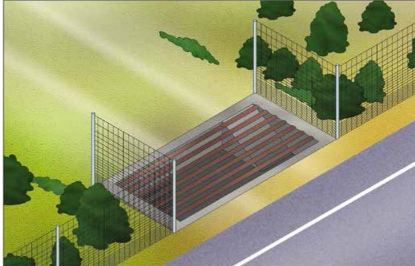
Figure 15.6 Diagram of a cattle grid for ungulates, with an interior escape ramp for animals that might accidentally fall into the trench beneath.
