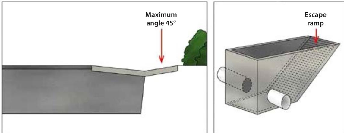
Figure 20.1. Diagram of an angled kerb and an exit ramp from a manhole or similar drainage infrastructure.
