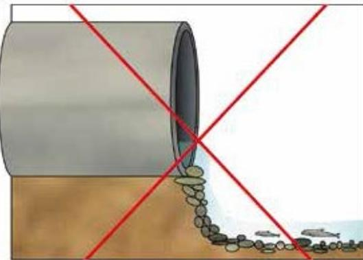
Figure 10.1. Top, culvert pipe adapted to facilitate aquatic fauna passage. Bottom, two alternatives that hinder upstream movement by fish due to shallow water or a significant height difference.
