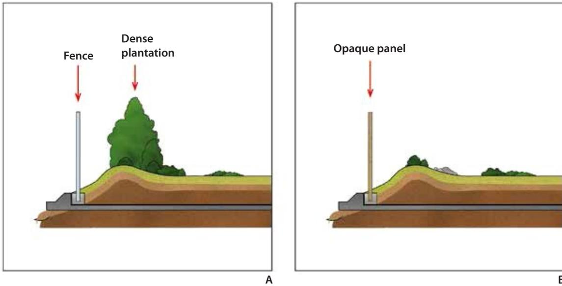
Figure 1.5. Details of an ecoduct section showing screening options. In Option A, a mesh fence is complemented with a dense vegetation screen to reduce disturbance by vehicle noise and lights. In Option B, more suitable in arid conditions, an opaque screen serves both purposes.
