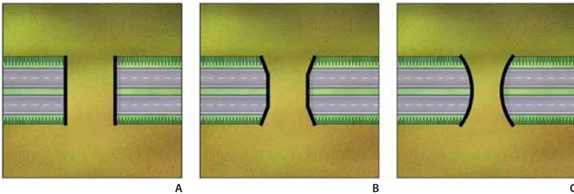
Figure 1.2. Alternative plans for ecoduct designs.
