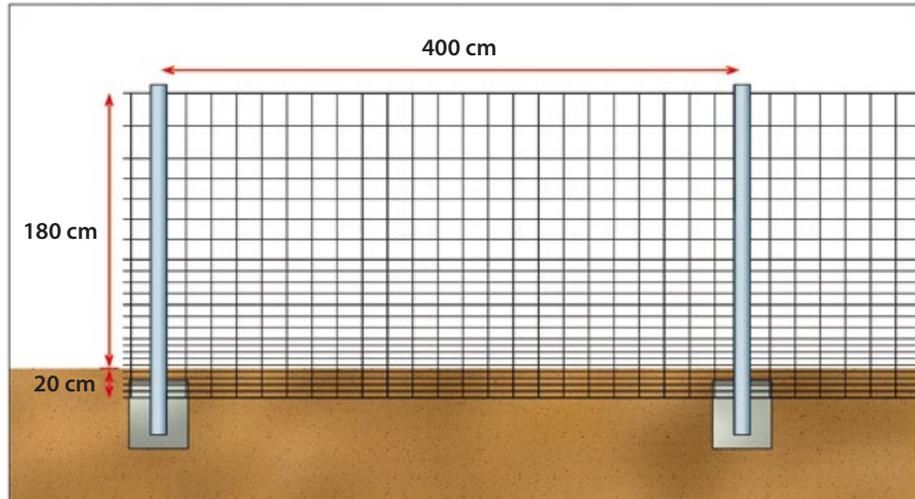
Figure 13.1. Diagram of a fence for large mammals.
