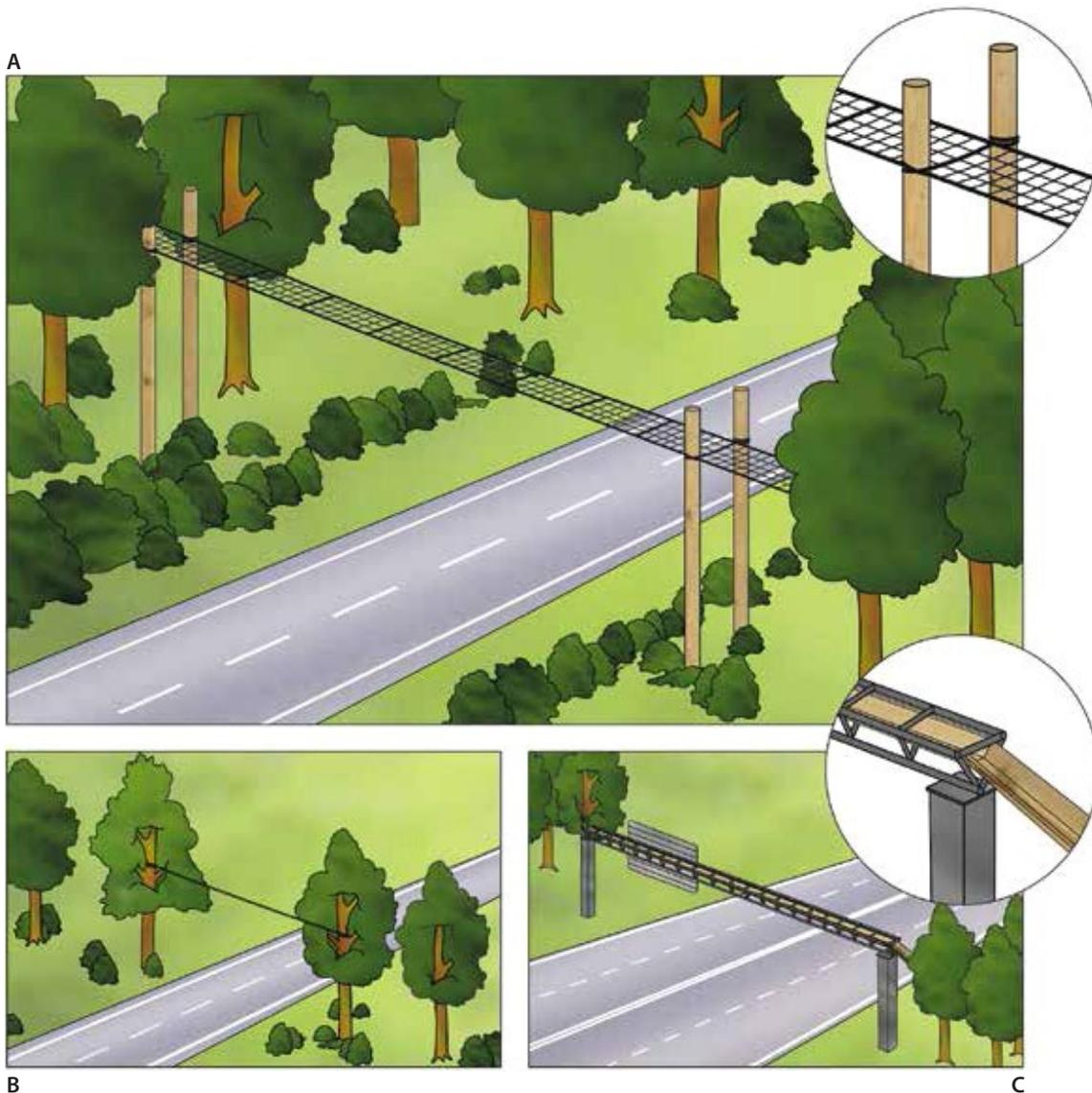
Figure 4.1. Diagram of different types of canopy bridges, depending on the road width. A: mesh bridge crossing. B: cable suspended between trees. C: platform for use as a wildlife crossing installed on road sign structures.
