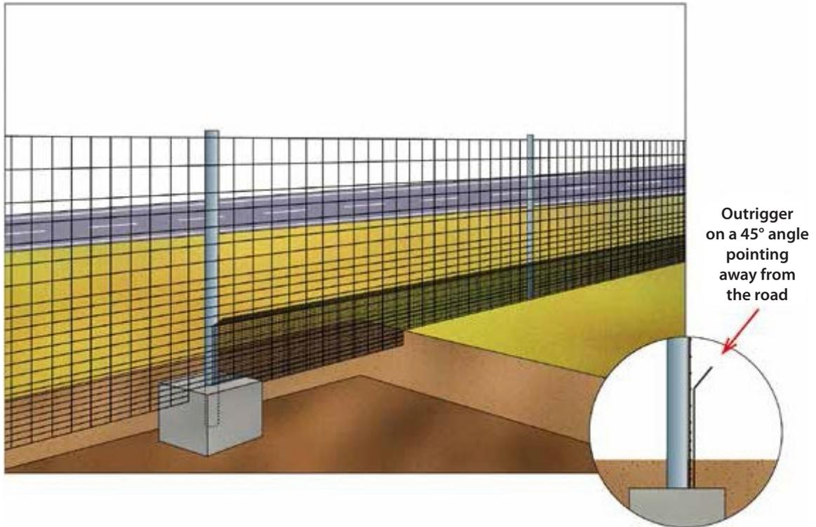
Figure 14.1. Diagram of reinforcement mesh, attached to the base of a fence for large mammals in order to prevent breaches by small vertebrates.
