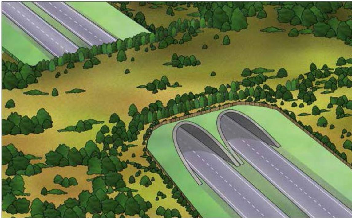
Figure 1.1. Diagram of an ecoduct.
