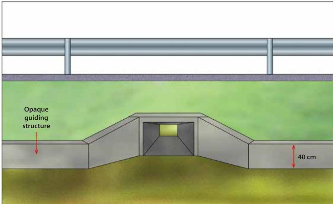
Figure 11.1. Diagram of an amphibian crossing.
