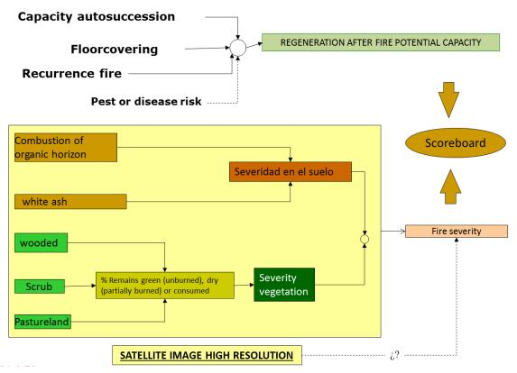
**Figure III-21.** Diagram used to assess fire severity, including field measures. The assessment can be complemented with indices obtained from remote sensing images (see Figure III-22).
