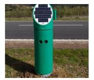
animals to run away. Lights are also visible to drivers that are also alerted. Beacons has a detection angle of  $160^{\circ}$ , and a detection distance of 13-17m. Distance between beacons is 20 m, therefore covering the whole sector.
