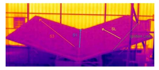
Figure 4.9. Schematic view of the Canyon Table of the Forest Fire Laboratory of the University of Coimbra indicating the position of the ignition line and the three directions S1, SL, and S3 along which the fire spread was analyzed.
