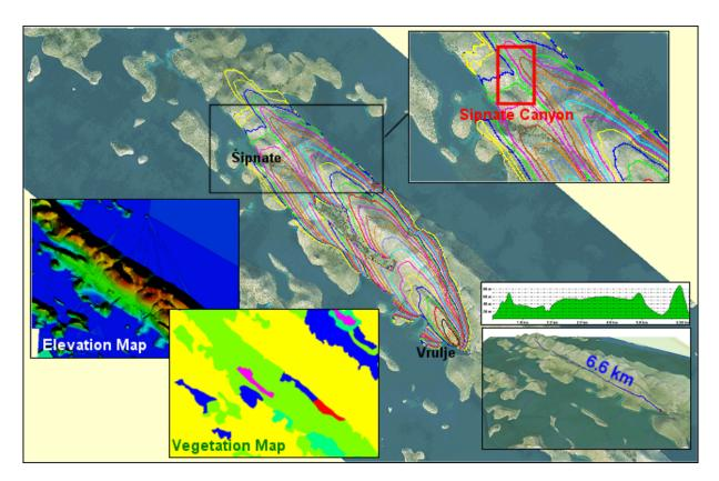
Figure 4.8. Fire spread simulation from the ignition point at Vrulje bay to the location of accident at Sipnate canyon based on Rothermel equations and adapted for Croatia at the University of Split. The dominant vegetation (light green) was modeled by Albini-Anderson category 1 (short grass), dead fuel humidity was 12% and average mid-flame wind speed 2.29 m/s.
