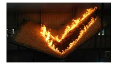
Figure 2.4. Experimental simulation of fire spread during the Guadalajara accident at the large Canyon Table DE4 of the Fire Laboratory of ADAI.
