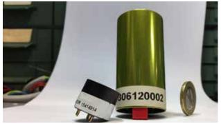
A **photo ionization detector** ionises volatile organic compounds and measures the resulting electrical current.
