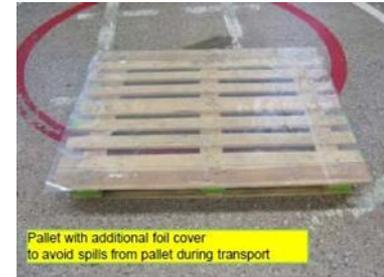
Pallet with additional foil cover to avoid spills from pallet during transport
