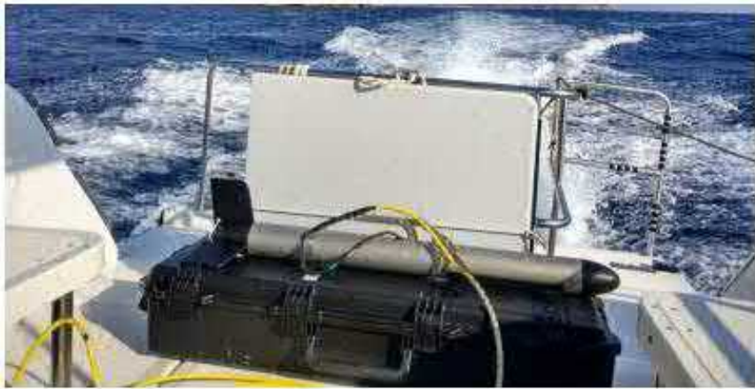
Fig. 21: Sonar de Barrido Lateral (SBL) PULSAR (Kongsberg Geoacustics)
