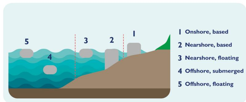
Depending on the size and orientation of the devices with respect to the swell, they can be classified as follows:
