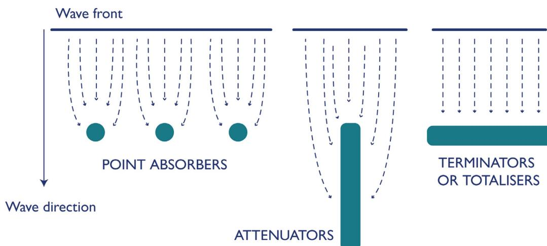
According to the wave-capture principle, which is the most commonly used classification of wave energy devices, they are classified as follows:
