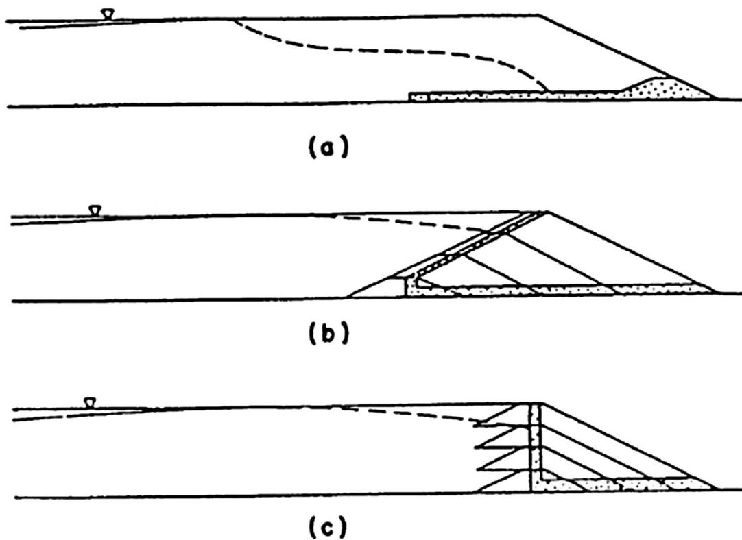
**Figure 45.** Bottom drainage systems in upstream, downstream and centerline mining tailing impoundments (IGME, 1986).
