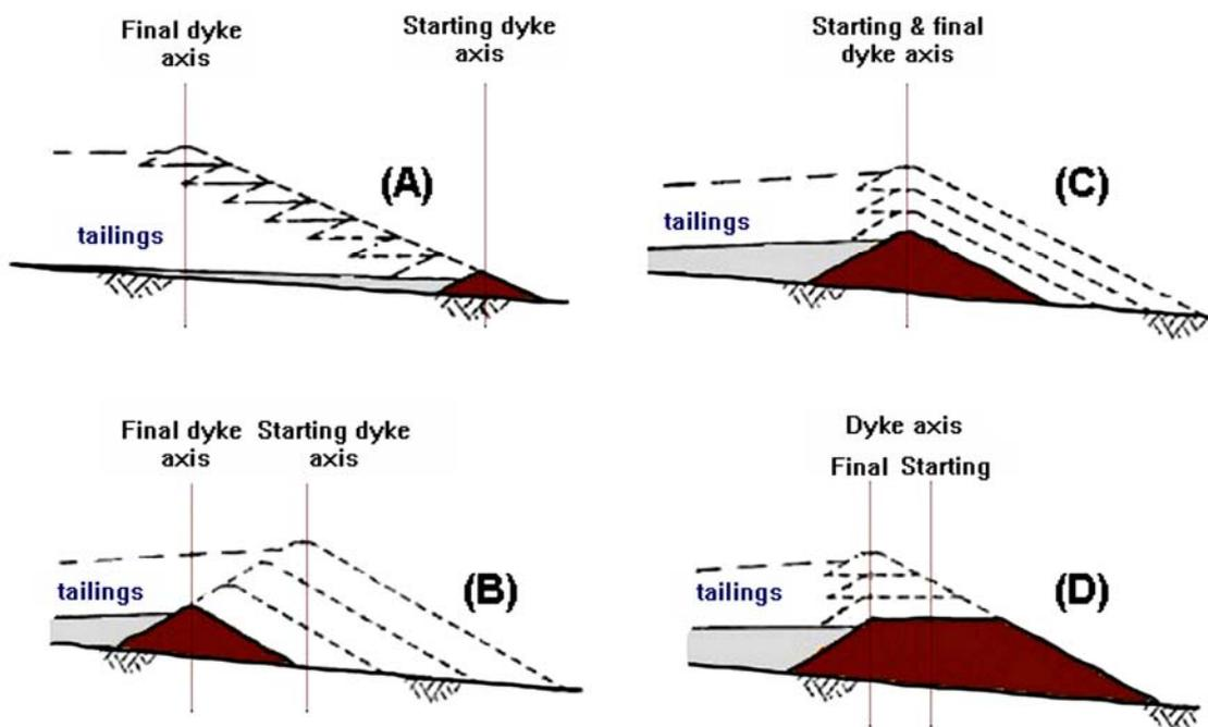
**Figure 37.** Types of mining tailing impoundments constructed through hydraulic filling using the mining waste themselves according to the regrowth system (modified from: Junghans and Helling, 1998). A) Upstream, B) Downstream, C) Centerline y D) Modified centerline.
