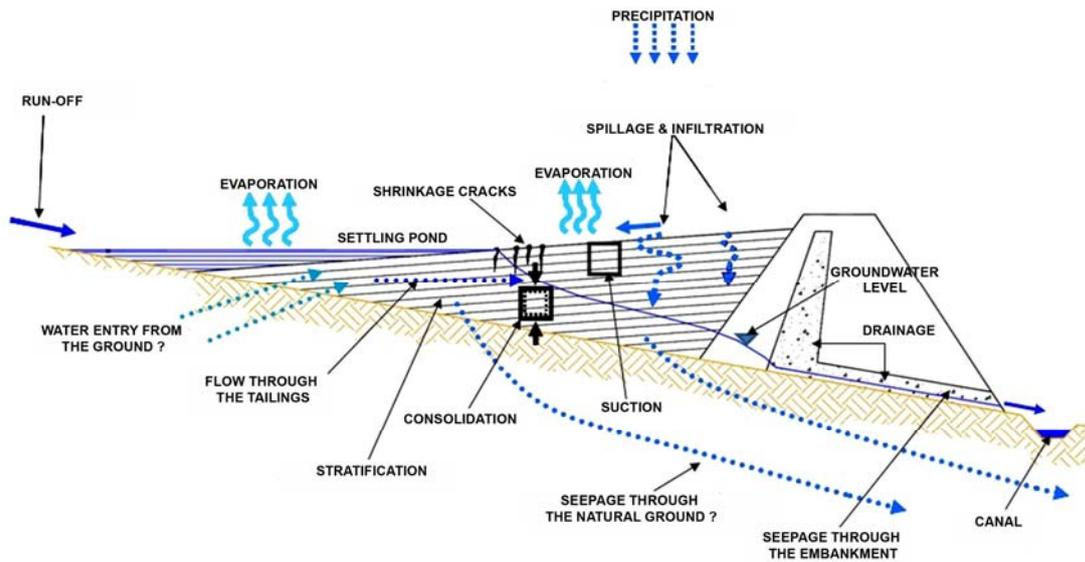
**Figure 43.** Schematic conceptual model showing the different components of an abandoned mining tailing impoundment (modified from Zandarin *et al.*, 2009).
