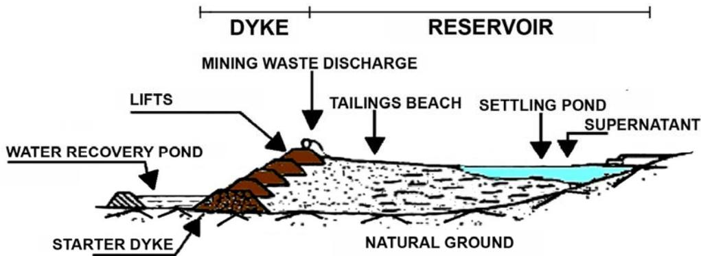
**Figure 36.** Mining tailing impoundment structure basic scheme (modified from: IGME, 1986).
