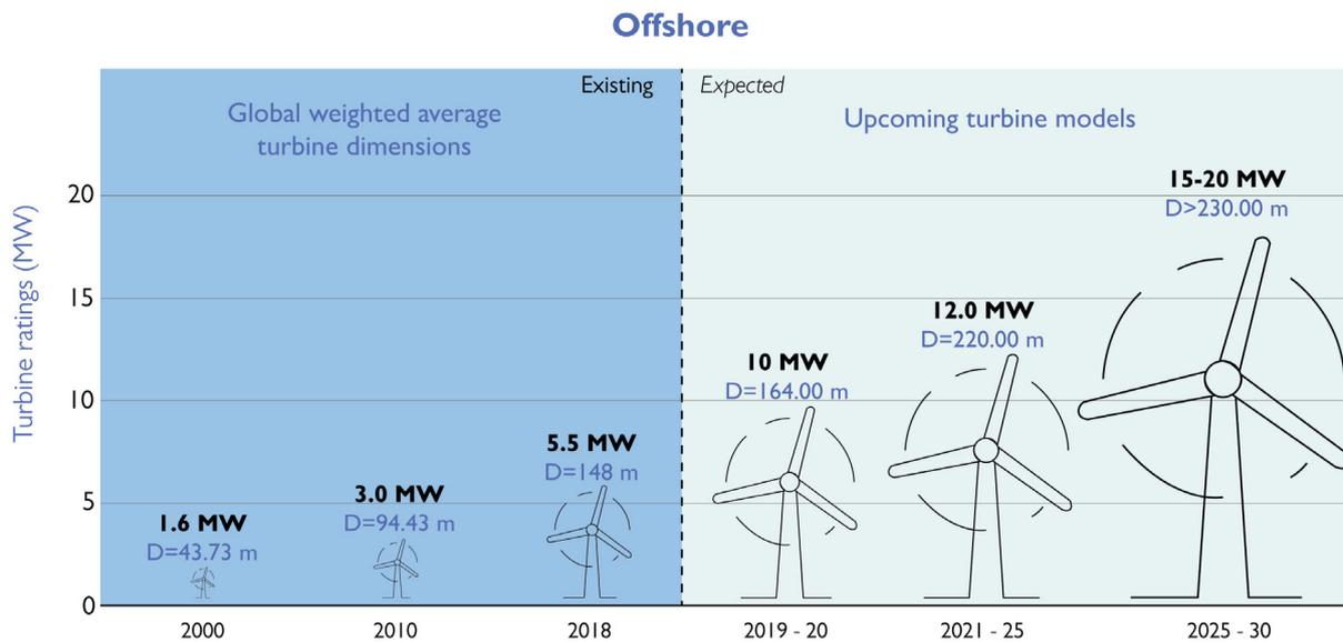
The average size of turbines used in offshore wind farms increased from 3 MW in 2010 to 5.5 MW for projects completed in 2018 (IRENA, 2019). New turbines of 10-12 MW will be able to achieve capacity factors well above 50% and prototypes under development will have an output of between 15-20 MW for offshore installation projects in 2025-2030.
