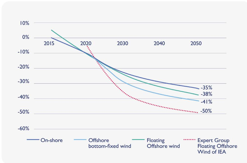
So far, this technology has already experienced a larger cost reduction than fixed-foundation offshore wind, and is expected to follow the same path from the current 180-200 €/MWh for small-scale pre-commercial projects, to 80-100 €/MWh in 2025 for the first commercial-scale projects using existing proven technologies. It is expected to reach 40-60 €/MWh by 2030 at commercial scale.
