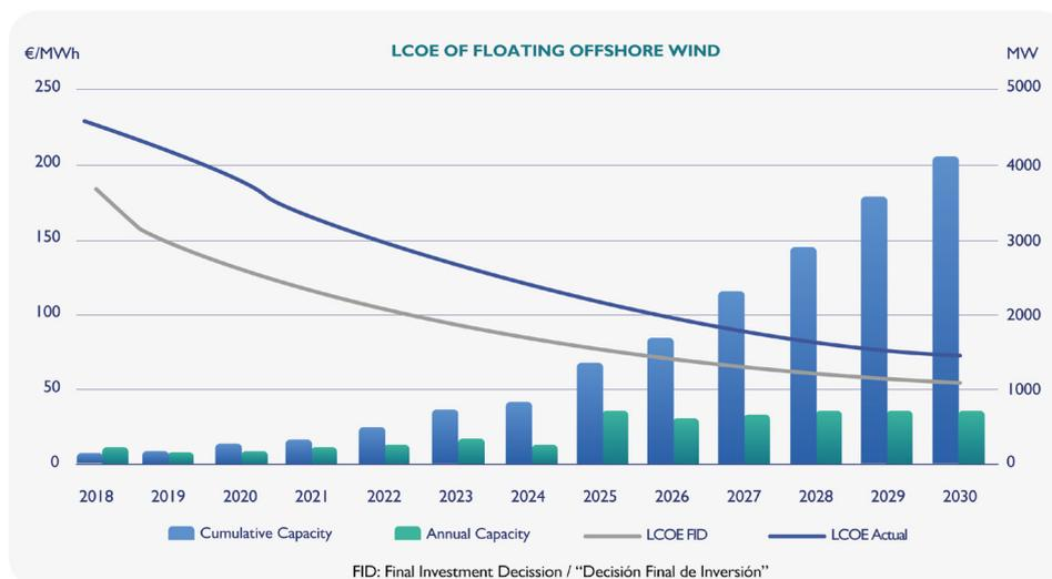
By December 2020, **compared to the aforementioned 29 GW of fixed-foundation offshore wind**, some 88 MW<sup>22</sup> of floating wind were installed globally, all pre-commercial, ranging in size from 2 MW to 30 MW, consisting of 1 to 5 machines of up to 8.4 MW unit power. Taking into account the planned projects, a **global cumulative floating wind capacity of approximately 350 MW would be reached by 2022**.
