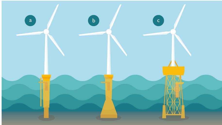
To date, all commercial offshore wind farms in service have been based on these fixed foundation typologies, having reached a cumulative figure of 29 GW<sup>14</sup> of offshore wind power in operation by the end of 2019. These fixed structures have been concentrated in water depths of less than 60 metres and close to shore, due to their lower cost. In Europe, the ‘monopile’ typology accounted for 80.5% of the foundations used for offshore wind turbines in 2020<sup>15</sup>.
