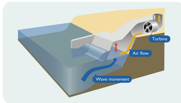
One of the distinguishing features of these converters is the significant cost savings that their construction and installation entails if it is carried out simultaneously with the execution of the coastal defence. As they are integrated into the infrastructure, the devices are not visible and do not pose any obstacle to coastal protection or affect the coastal landscape.
