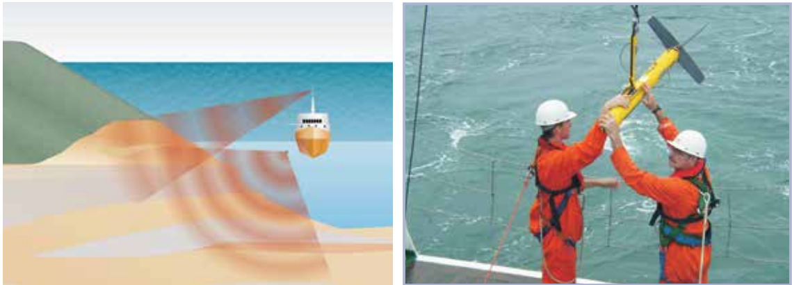
Figure 7.74 Over water methods – side-scan sonar 'towfish' (courtesy Fugro)
