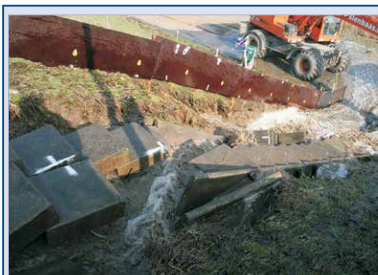
Figure 4.14 Testing of resilience on levee with staircase, the Netherlands (courtesy Y Provoost, RWS, the Netherlands )
