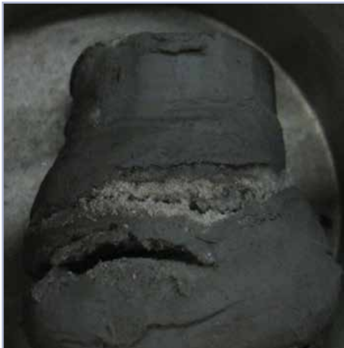
Figure 9.94 Sample of clay with sand lenses (courtesy Mike Wielputz, USACE)
