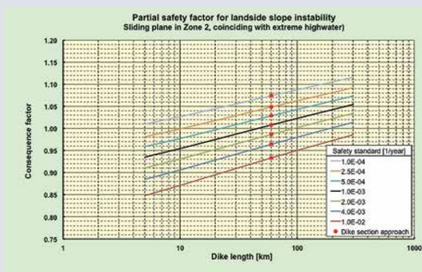
Figure 9.64 Required stability factors for zone 2 and P_{f,inst} = 0.1 (dike ring approach) (courtesy Harry Schelfhout, Deltares)
