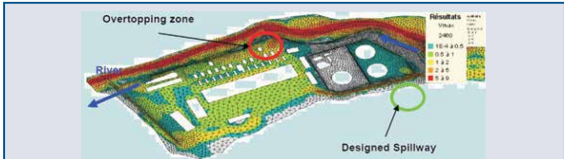
Figure 8.151 Example of flood map showing maximum flow velocities due to levee overtopping calculated from 2D finite element software (Telemac) for which the computational mesh is shown (EGIS Eau for EDF PEI, 2009)
