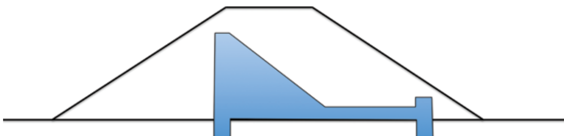
Figure 9.114 Reinforced concrete spillway (after Degoutte et al , 2012)
