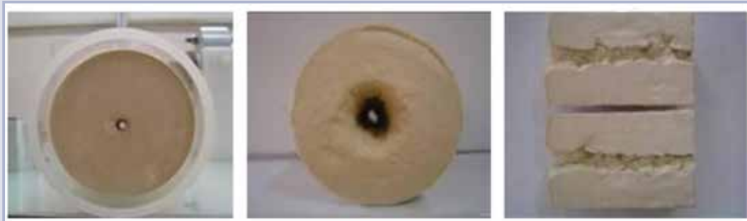
Figure 8.66 Example of enlargement of initial hole by erosion on white kaolinite sample, sample before the test (a), sample after the test (b), and longitudinal section of the sample after the test (c) (Benahmed and Bonelli, 2012)
