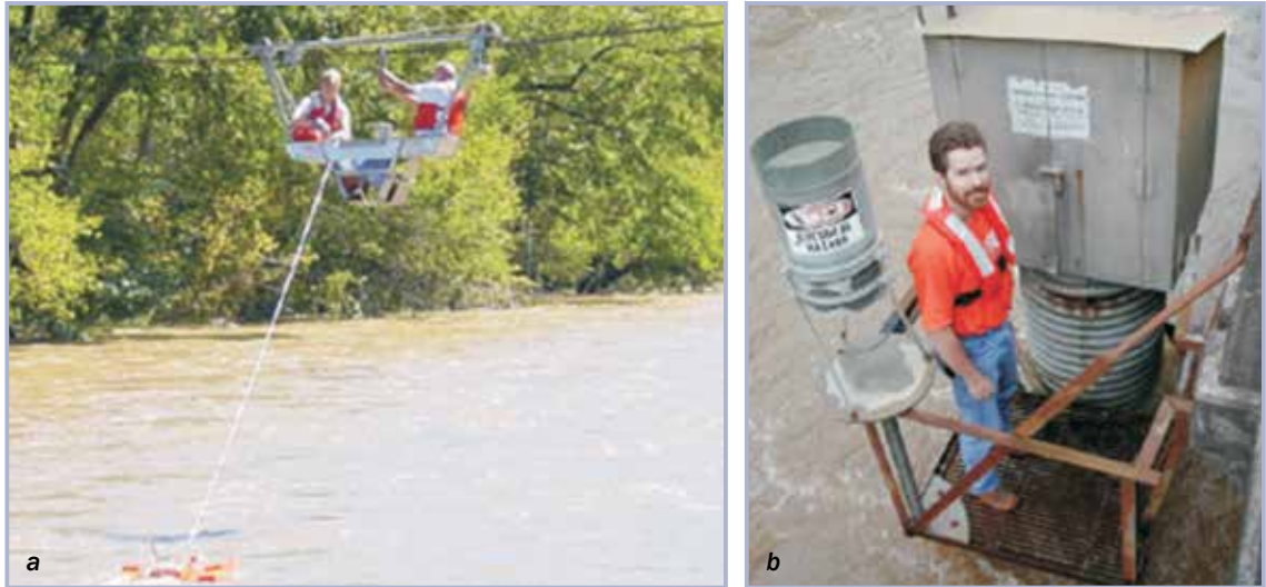
Figure 7.19 Direct flow measurements by hydrographers using Acoustic Doppler Current Profiler (ADCP) (a), field data collection platform for stream gauge and precipitation (b) (courtesy USGS)
