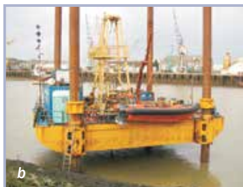
Over water drilling platforms (a) floating pontoon, (b) jack-up rig, and (c) drilling ship (courtesy Fugro)
