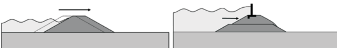
Figure 3.186 Translational sliding of a levee on a soft soil foundation or in the levee body (courtesy Y Deniaud, CETMEF)
