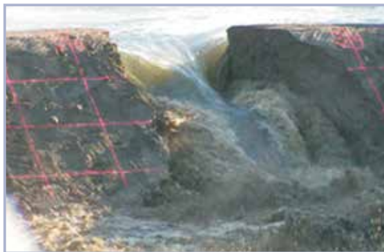
a Sediment erosion by turbulent flow along base of breach sides
