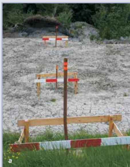
Figure 10.66 Settlement plates in the Lake Marken levee improvement project (courtesy Fugro)
