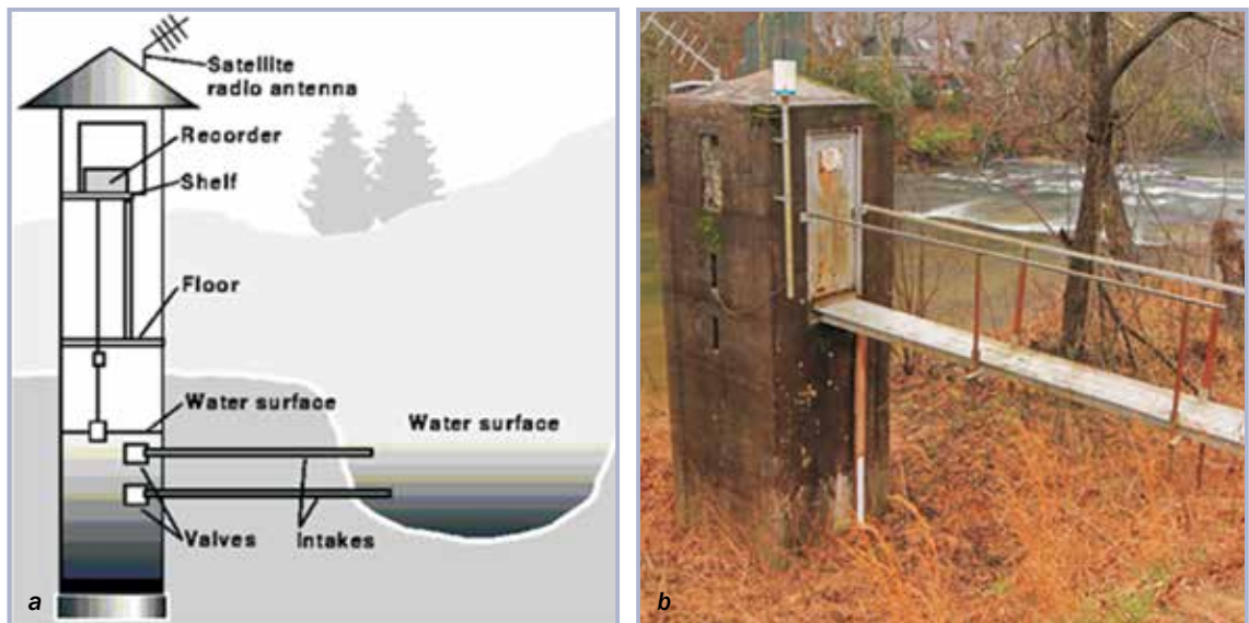
Figure 7.20 Schematic (a) and photograph (b) of a typical river gauge installation (courtesy USGS)
