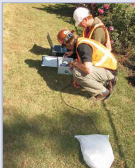
Figure 10.65 Vibration monitoring, Sacramento, USA
