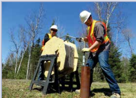
Figure 7.79 Measurand ShapeAccelArray (SAA) (courtesy Measurand Inc)
