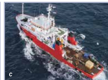
Over water drilling platforms (a) floating pontoon, (b) jack-up rig, and (c) drilling ship (courtesy Fugro)
