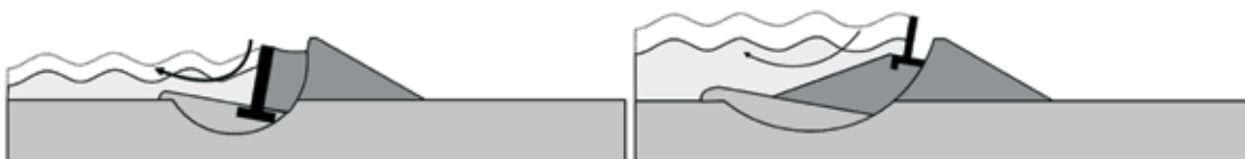
Figure 3.185 Deep rotational sliding affecting a waterside wall of a levee (courtesy Y Deniaud, CETMEF)
