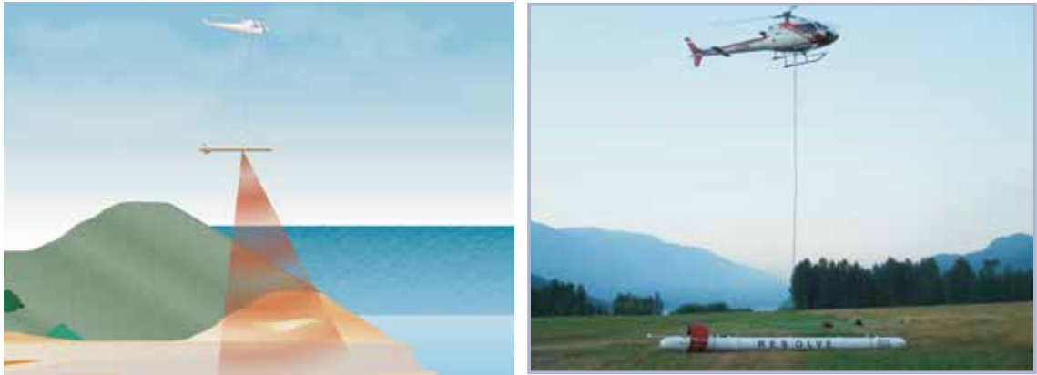
Figure 7.75 Airborne methods – frequency domain EM measurement (courtesy Fugro)
