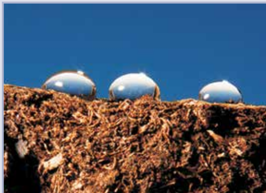
Figure 4.46 Examples of water-repellent peat levees (courtesy of E Eisen (a) and B James (b))
