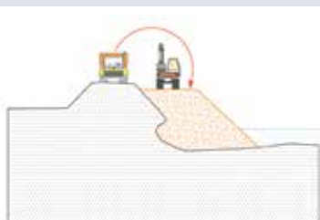
Figure 10.60 Truck supplies rock to excavator to create berm
