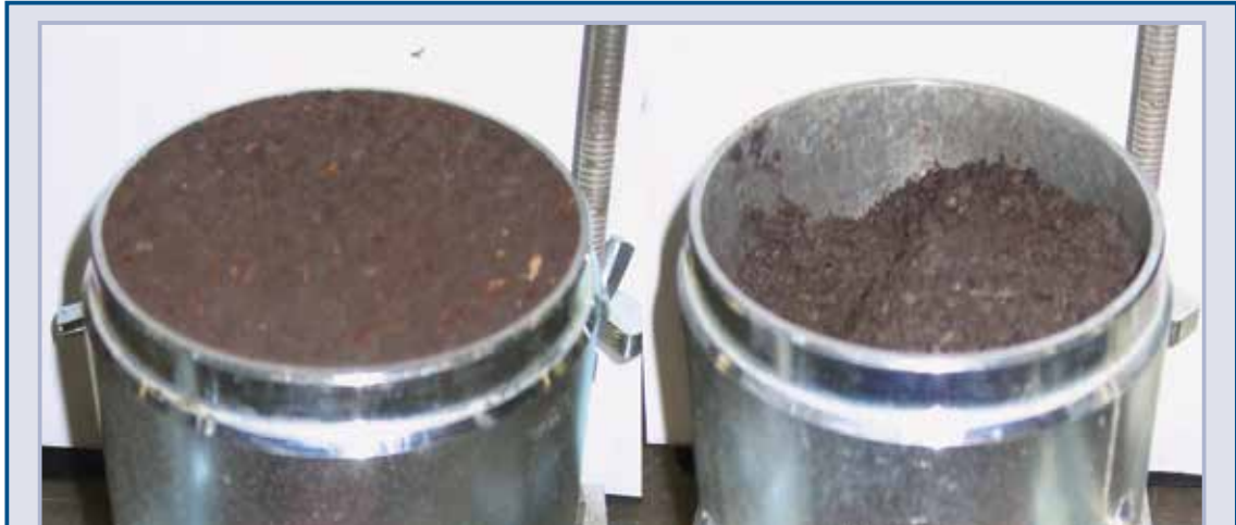
Figure 9.86 Determining erodibility of organic clay; photographs taken before and after application of a water jet (courtesy Mike Wielputz, USACE)
