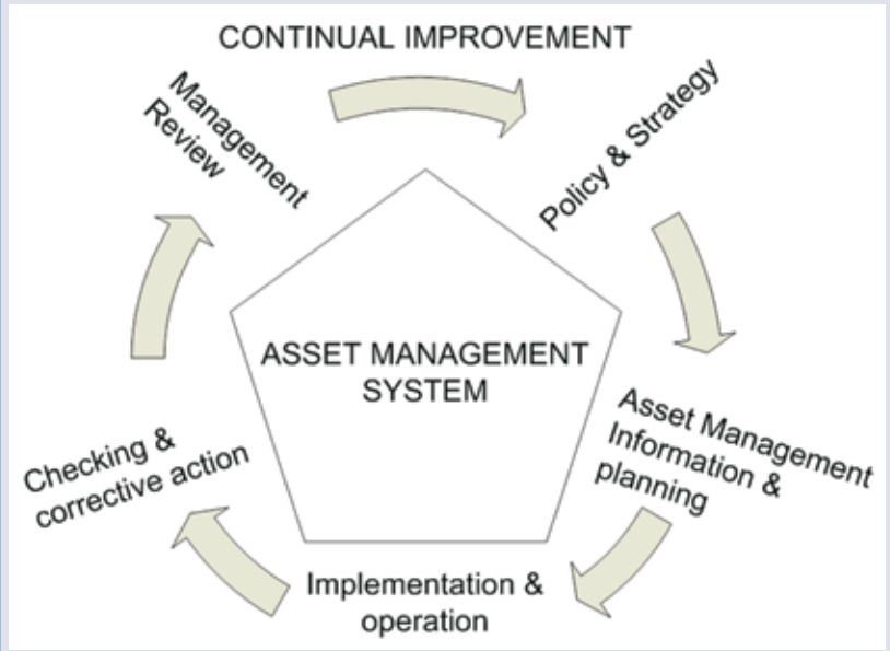
Figure 2.13 The asset management system in the UK, plan-do-check-act cycle (from BSI, 2008)
