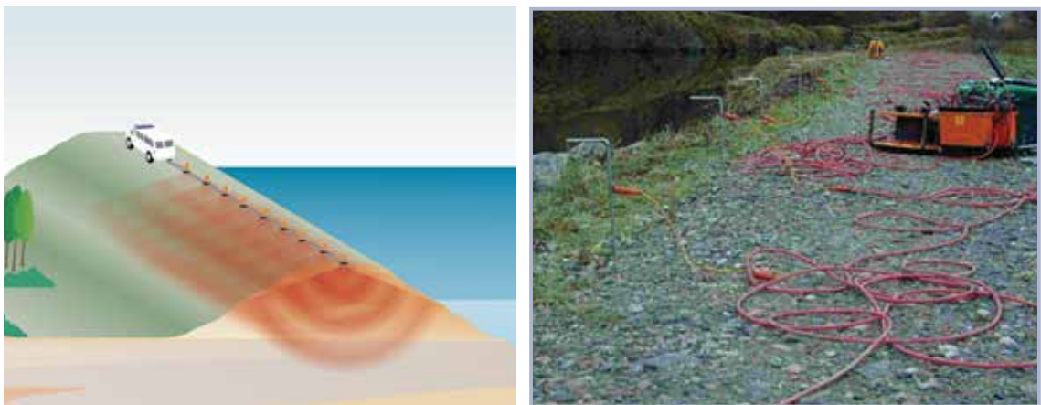
Figures 7.73 Surface methods: electrical resistivity tomography (courtesy Fugro)
