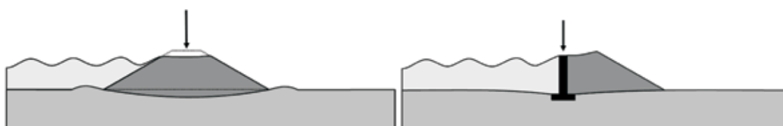
Figure 3.187 Settlement of a levee on a soft soil foundation (courtesy Y Deniaud, CETMEF)
