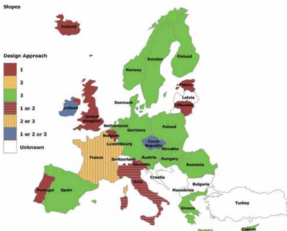
Figure 9.61 Design approaches adopted by different European countries for design of slopes and embankments (Bond, 2013)
