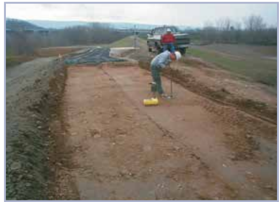
Figure 10.25 Laboratory technician using a nuclear density gauge to measure field density after compaction (courtesy USACE)
