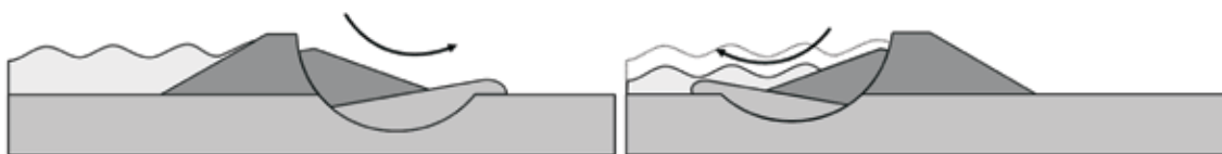
Figure 3.184 Deep rotational sliding of a levee (courtesy Y Deniaud, CETMEF)
