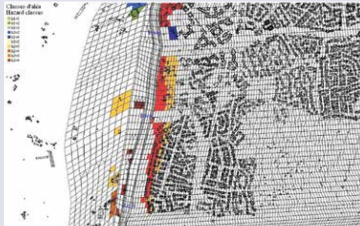
Figure 8.150 Flood map showing high risk areas due to levee failure calculated from 2D hydraulic model
