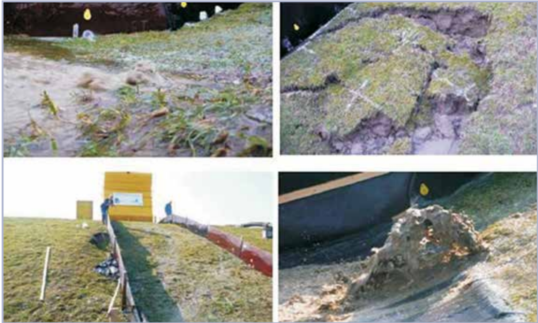
Figure 8.50 Recent Dutch studies into grass performance under wave overtopping, using the wave overtopping simulator (Morris et al, 2012a)
