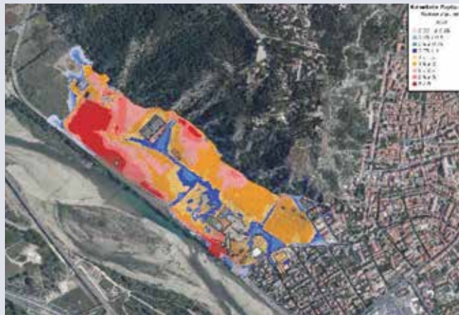
Figure 8.143 Example of zoning of water depths 30 minutes after a levee breach in an urban area (Th. Monier, Sogreah, 2011)
