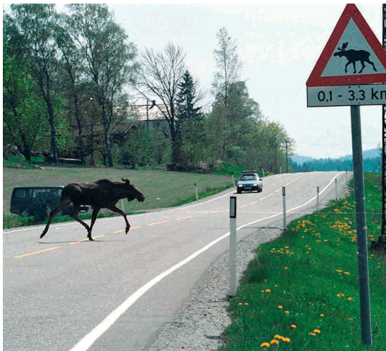
Figure 7.87 - A moose warning sign in Norway. Such warning signs are not very effective, because drivers get used to them. (Photo by S. Persson, Østlandets Blad)
