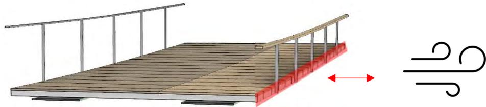
$$\frac{F_{wY \text{ tablero}}}{A_{ref}} = 1.209 \frac{kN}{m^2} \cdot c_{f,y} = 1.564 \frac{kN}{m^2}$$
